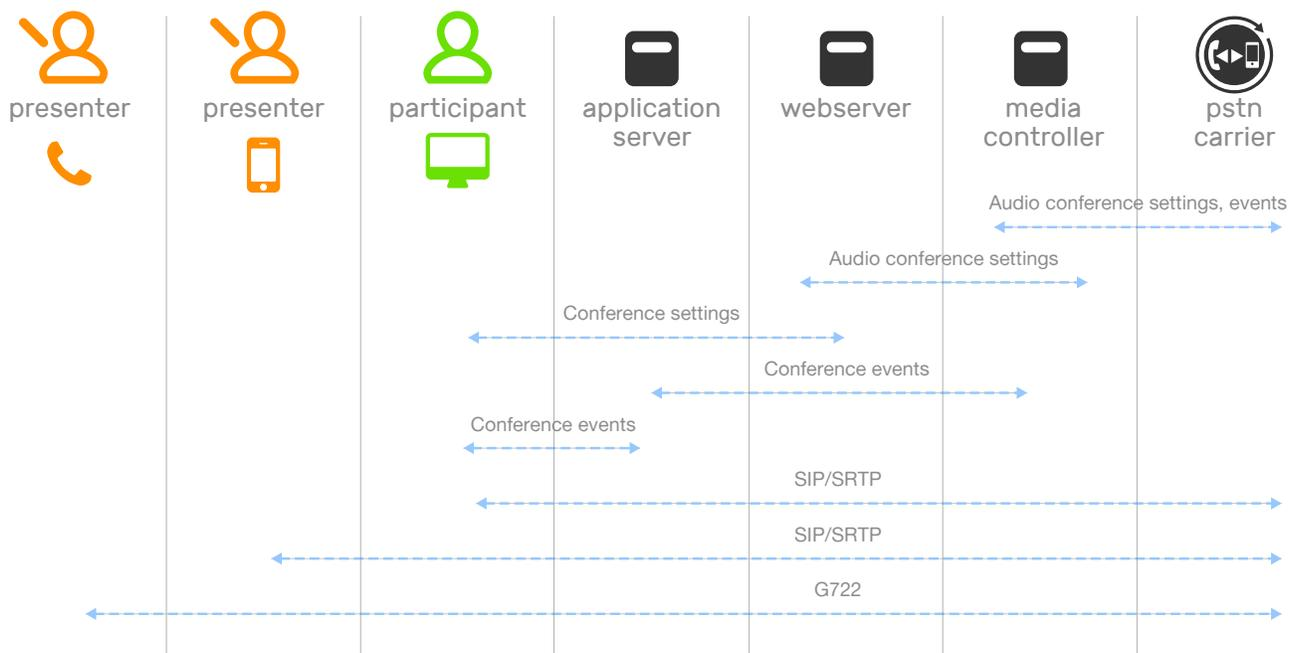
**join.me** audio is based on the Voice over IP (VoIP) using the secure SIPS standard to facilitate communication between the computer and the audio infrastructure. In some network environments, this may require the following ports and IP ranges to be opened in the firewall:
