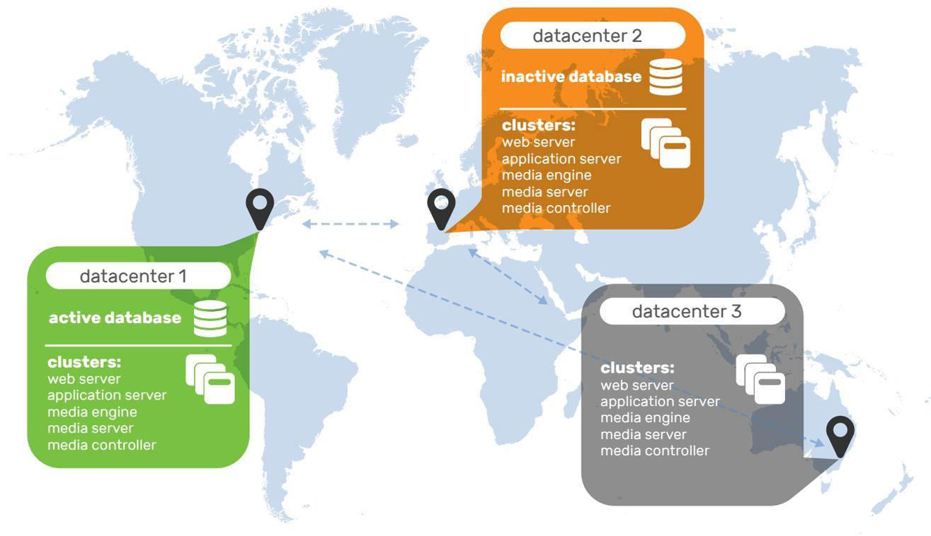
Datacenters are connected with a VPN mesh, meaning, for example, that if Datacenter #1 were to lose direct connection to Datacenter #2 it would communicate instead through Datacenter #3. Inter-datacenter communication is essential because only one datacenter hosts an active **join.me** database. In the illustration above this is Datacenter #1.
